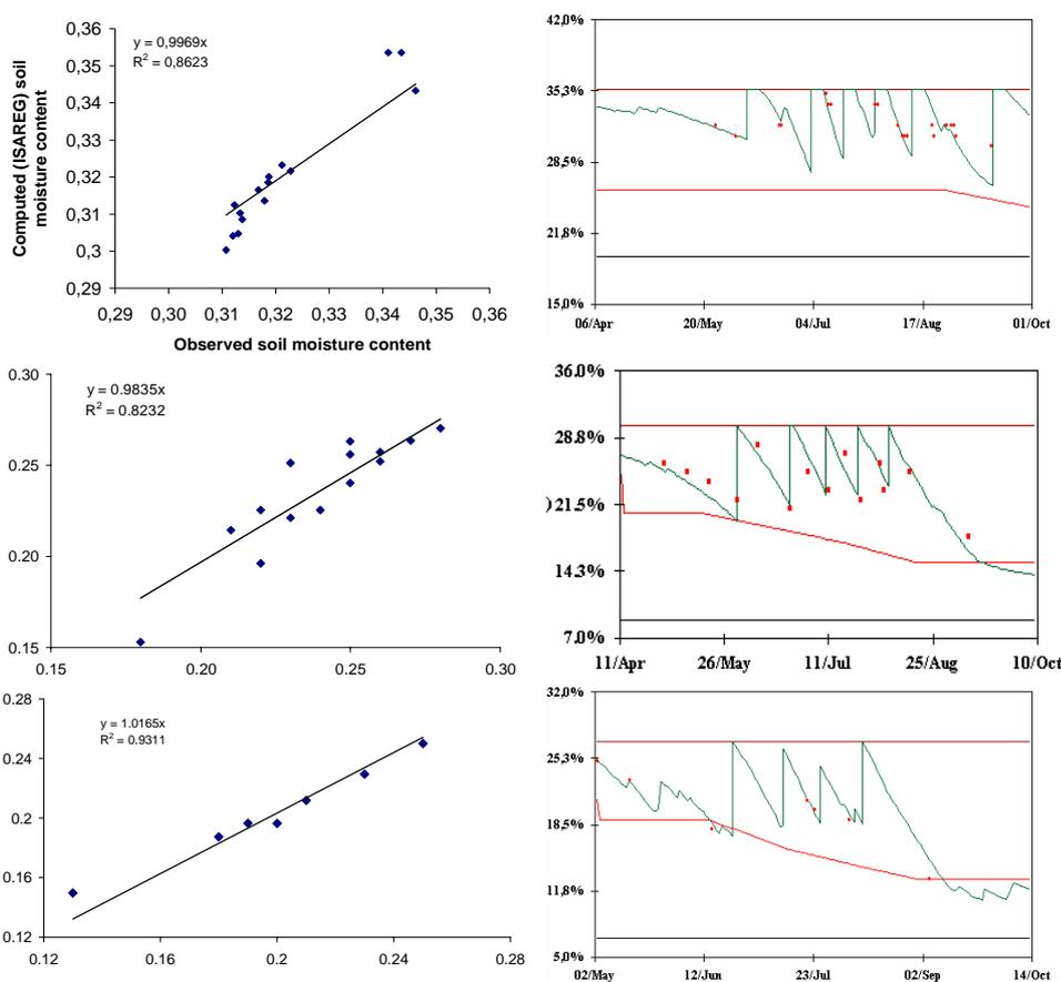
Fig. 19. Comparison between observed and simulated soil water content for cotton: a) and b) at the “Azizbek-1”, 2001 (field #13 and 5); and c) at “Sandik” farm, 2003.
