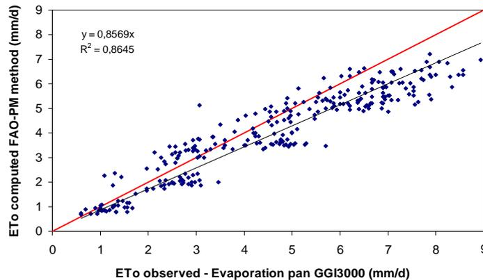
Fig. 14. Comparison between observed average 10-day GGI3000 pan evaporation and computed FAO-PM reference evapotranspiration ( $mm\ d^{-1}$ ) for Fergana, 1970-2003.
