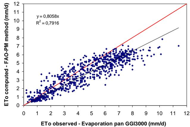
Fig. 15. Comparison between observed daily GGI3000 pan evaporation and computed daily FAO-PM reference evapotranspiration in Fergana oblast (2001-03).
