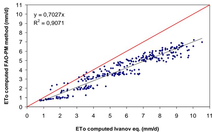
Fig. 16. Comparison between FAO-PM reference evapotranspiration and ET computed with Ivanov's formula for Fergana oblast for the period 1970-2003 (April-November).
