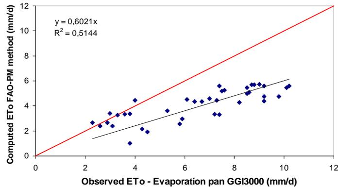
Fig. 17. Comparison between observed (evaporation pan GGI3000) and computed reference evapotranspiration (FAO-PM), for Osh oblast, 2001-03.
