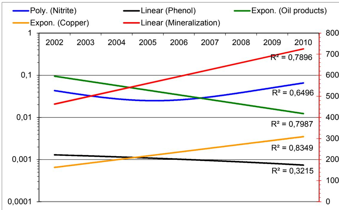
Fig. 11: Trends for the pollution with Nitrite, Phenol, Oil products, Copper and for the Mineralization in the Uzbek part of the Zarafshon (in mg/l, the mineralization is displayed on the secondary axis)
